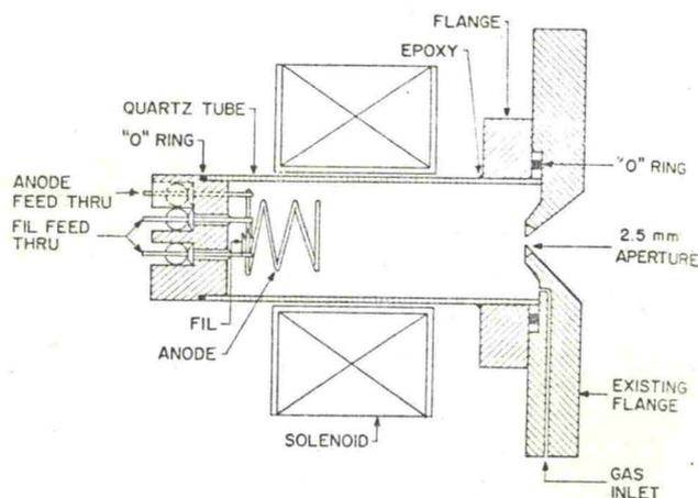
FIG. 1. Schematic drawing of the oscillating electron source.
